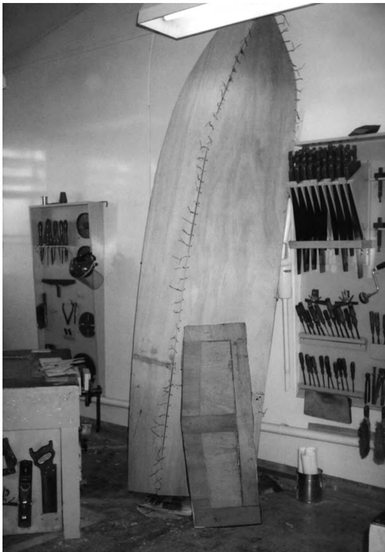
Fig 3.8: The ply components laced together.
