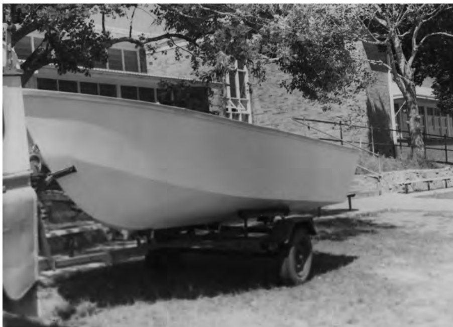
Fig 1.3: This boat was made from 6mm marine ply, stitch and glue method with F.R.P. sheath.
