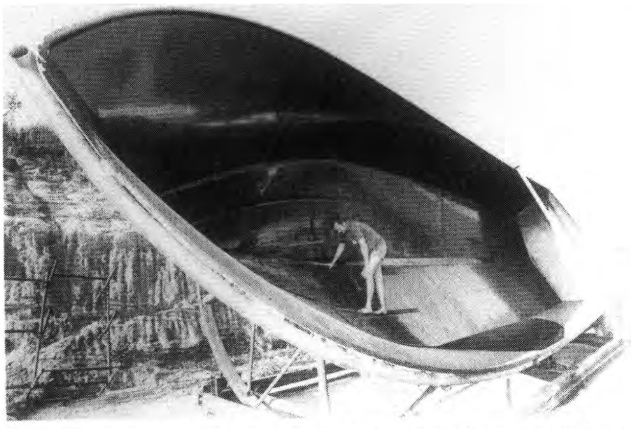
Fig 1.9: A 12.8 metre mono hull mould (Photo courtesy Sunshine Coast Kevlacat)
